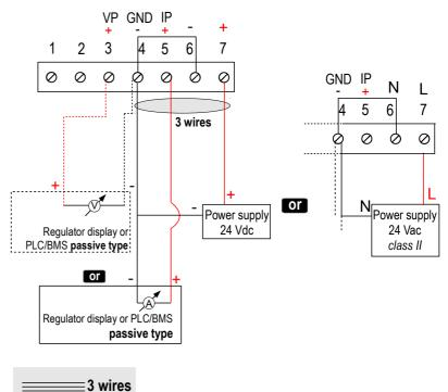
For  $\mbox{CP116-PO}$  and  $\mbox{CP116-PN}$  models with 4-20 mA output – passive :
