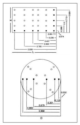
Simplified plan according to NF.X10.112 norm of the measurement points following the "Log. Tchebycheff" method.
